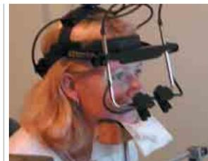
To track a subject's eye movements, Gilchrist employs sophisticated eye-tracking equipment which uses an infrared video system sampling at 500 Hz, with a spatial accuracy of 2mm on the computer screen.
